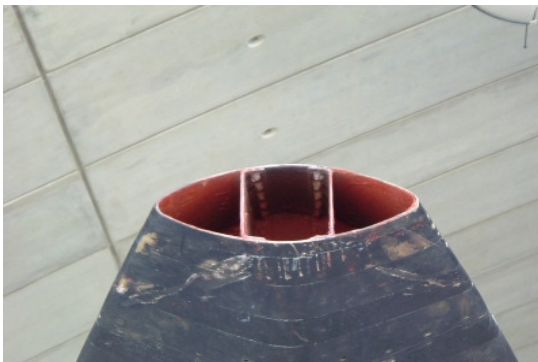
Fuel Dump at the end of the 'boat' tail.
