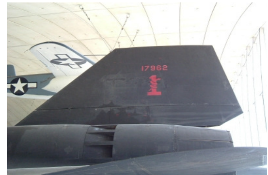
All moving Rudders canted inwards at 15 degrees. Note the tertiary doors - these closed above Mach 1.5.
